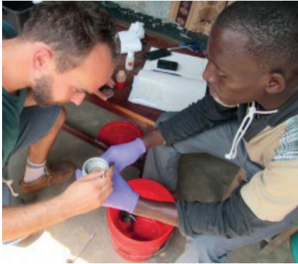
Figure Mike Coto showing a local student Jonathon some biological water testing methods using an Oxfam Del Agua kit, in the town of Vingunguti, in the Ilala district of the Dar es Salaam Region
