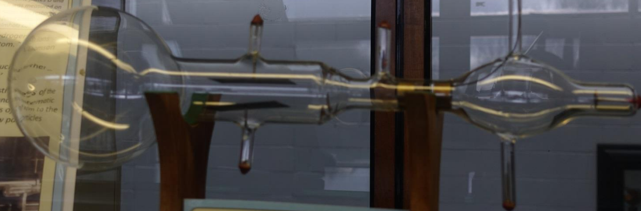
Replica of the gas discharge tube with which Thomson discovered the electron, made by Richard Smith, a former glass-blower in the Cavendish Laboratory.
