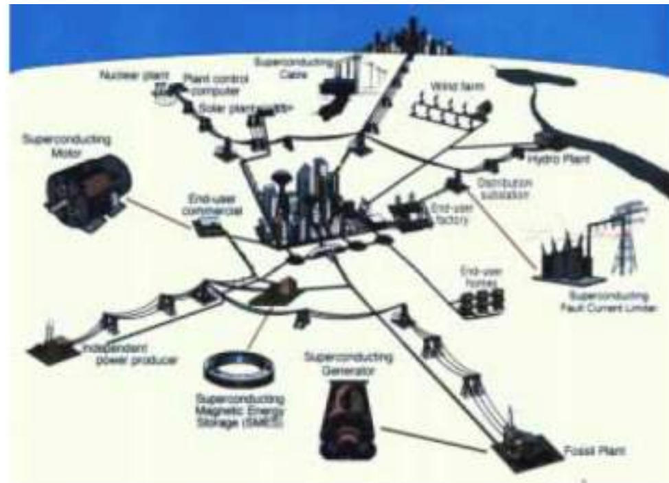
Fig. 1.1. Superconductivity in the electric power system of the future, with widespread use of superconducting generators and motors, fault-current limiters, underground transmission cables, and superconducting magnetic energy storage (Blaugher 1995).
